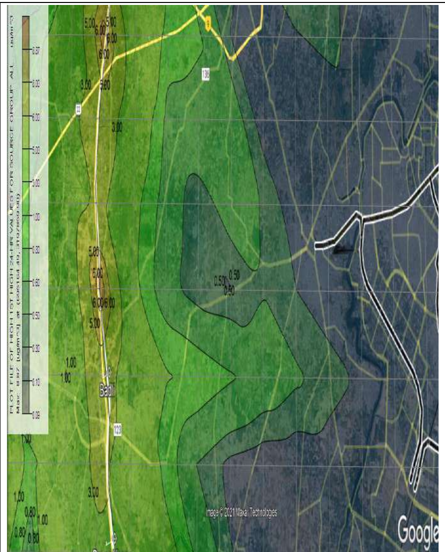
PM 10 INCREMENTAL GLC AT BADLI STATION LOCATION
