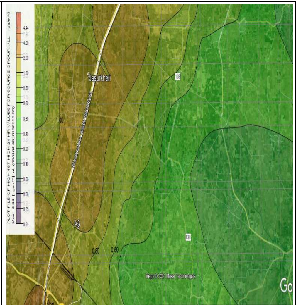
PM 2.5 INCREMENTAL GLC AT JASURKHERI STATION LOCATION
